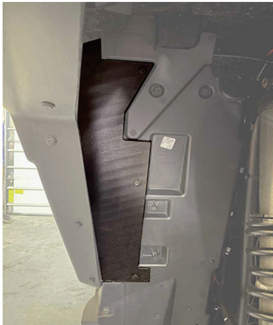
Figure 1: Line up the holes in the block off with the factory-drilled holes
